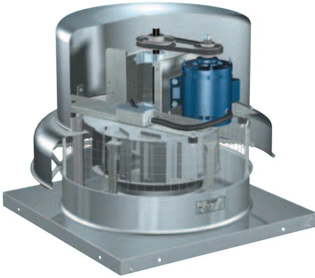
Spun aluminum downblast exhaust fans shall be belt drive-type. These fans are specifically designed for roof mounted applications exhausting relatively clean air. Performance capabilities range up to 44,700 cfm (75,946 m<sup>3</sup>/hr) and 2.5 in. wg (623 Pa) of static pressure. The maximum continuous operating temperature shall be 180°F (82°C). Model GB fans are available in twenty sizes with nominal wheel diameters ranging from 11 to 54 inches (279 to 1372 mm) (071-540 unit sizes).
