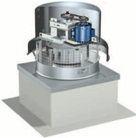
Spun aluminum downblast exhaust fans shall be belt drive-type. These fans are specifically designed for roof mounted applications exhausting relatively clean air. Performance capabilities range up to 44,700 cfm (75,946 m<sup>3</sup>/hr) and 2.5 in. wg (623 Pa) of static pressure. The maximum continuous operating temperature shall be 180°F (82°C). Model GB fans are available in twenty sizes with nominal wheel diameters ranging from 11 to 54 inches (279 to 1372 mm) (071-540 unit sizes).
