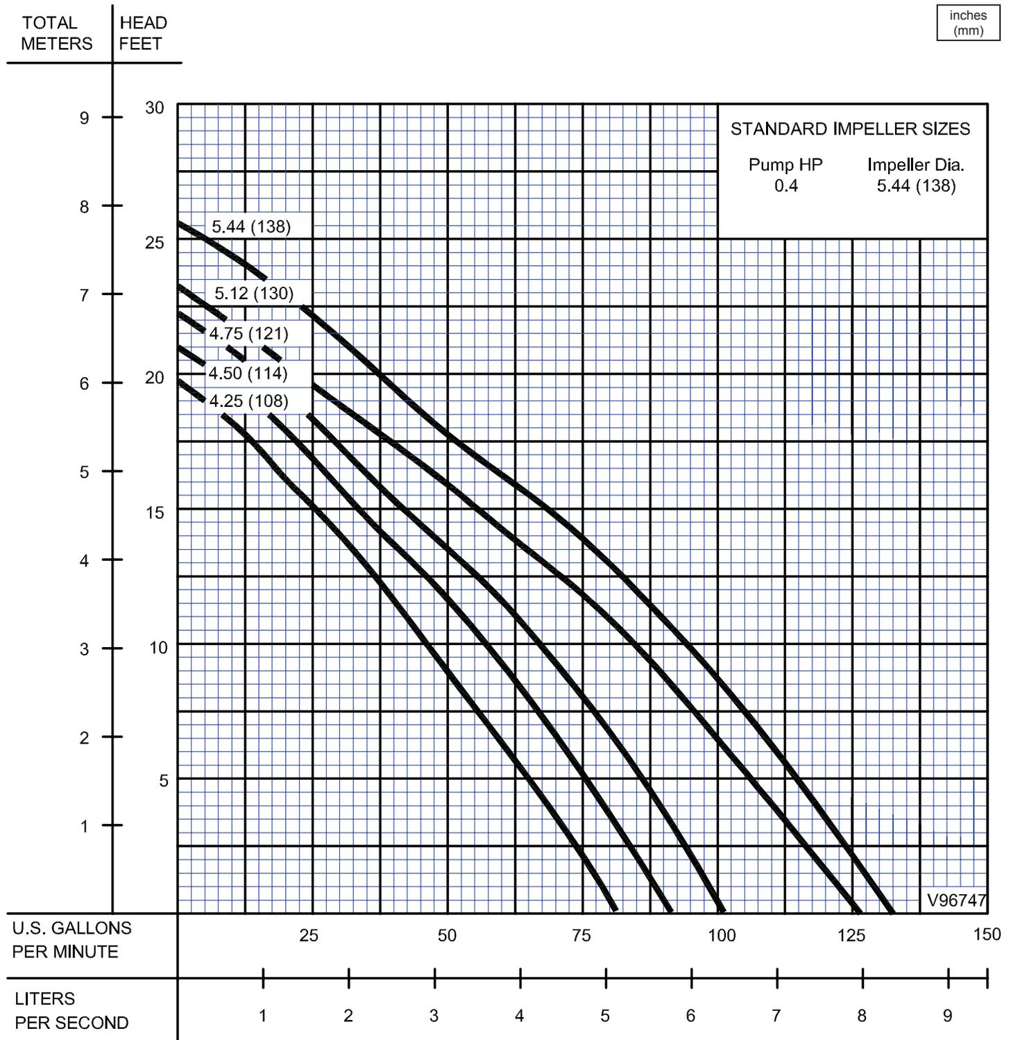
Testing is performed with water, specific gravity 1.0 @ 68° F @ (20°C), other fluids may vary performance
